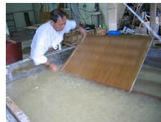
Fig. 12 Dipping the right side of the mould into vat
