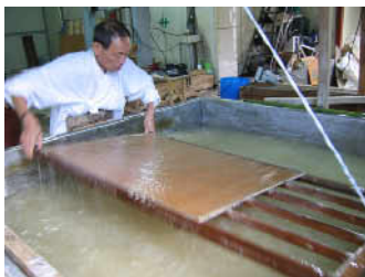
Fig. 11 Swinging mould to remove excess fibers
