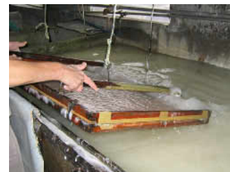
Fig. 16 Excess fibers are tossed off top of mould
