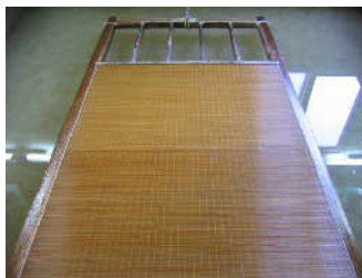
Fig. 2 Mould and screen for Webal method
