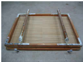
Fig. 13 Mould and deckle for Ssangbal method
