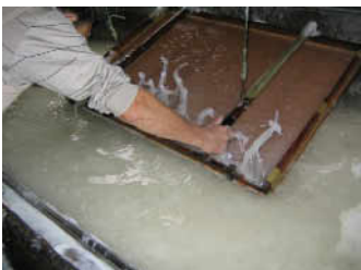
Fig. 14 Scooping fibers onto mould with deckle
