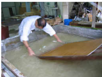
Fig. 8 Initial dip of Webal method of sheet forming
