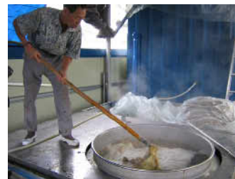
Fig. 3 Cooking white bark with alkali to remove non-cellulosics
