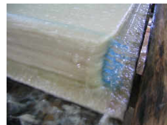
Fig. 19 String used to separate sheets on post of wet sheets
